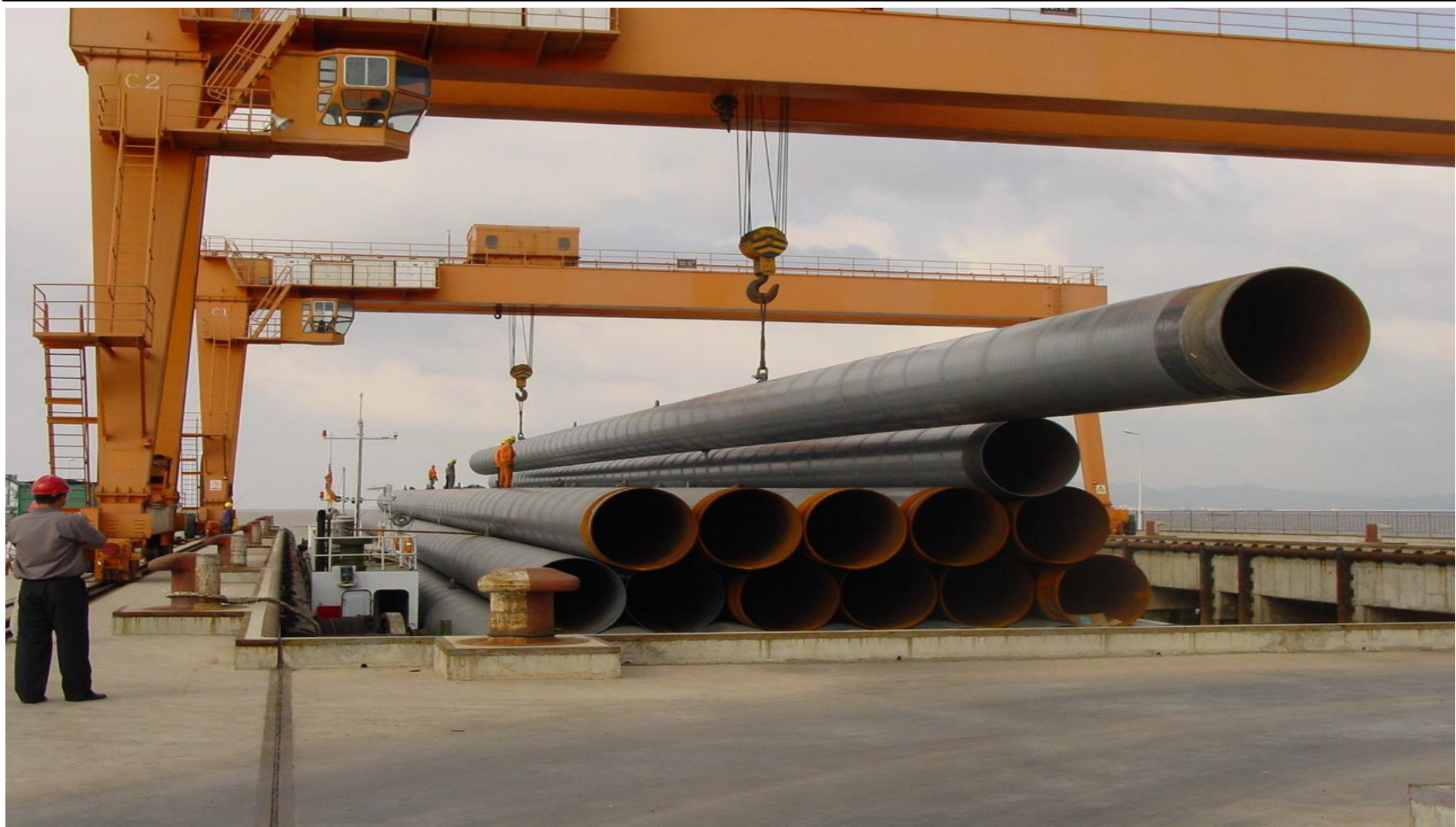
3LPE COATED EXTRA LENGTH PIPE PILING
