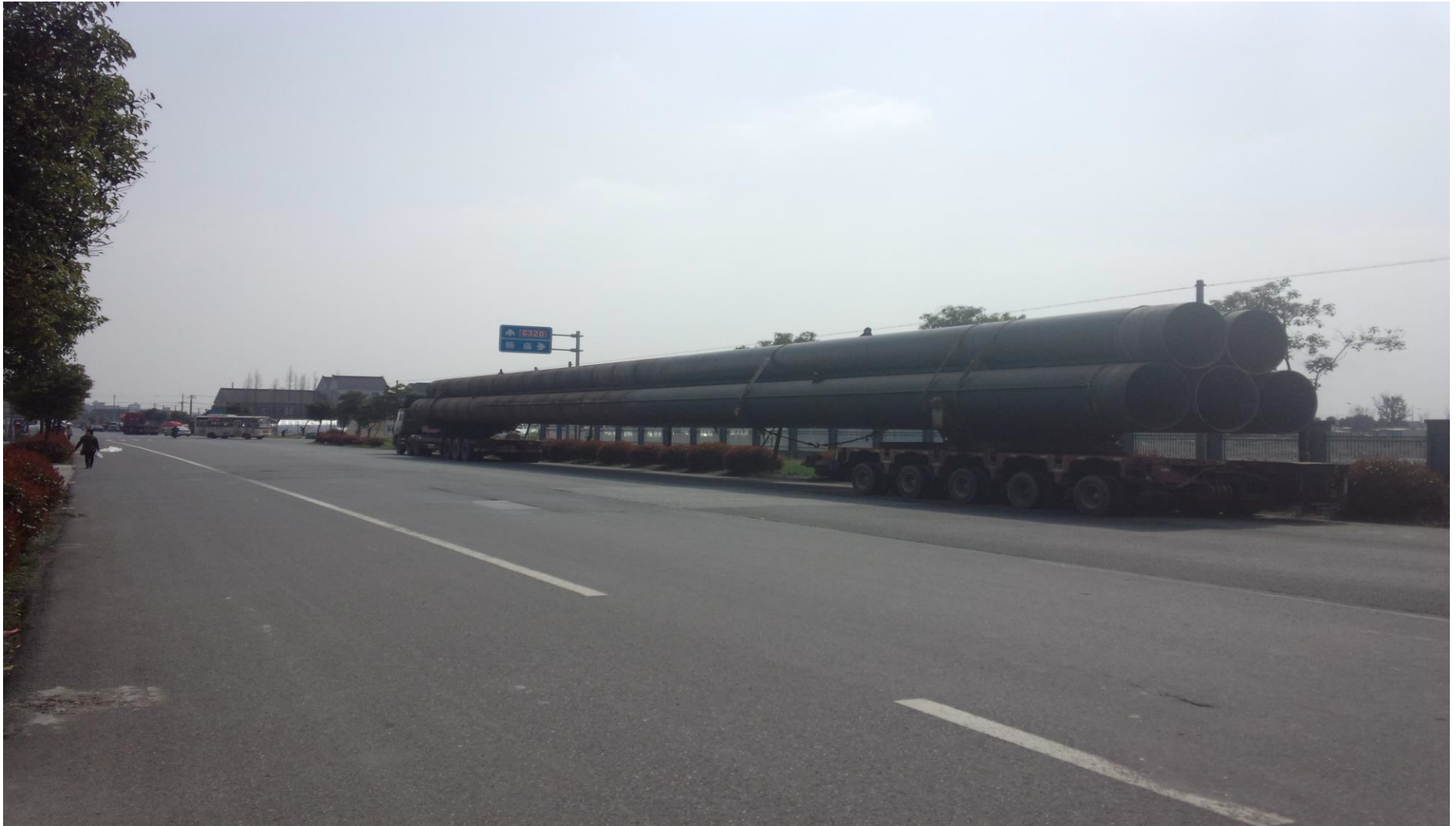
TRUCK TRANSPORTED EXTRA LENGTH PIPE PILING
