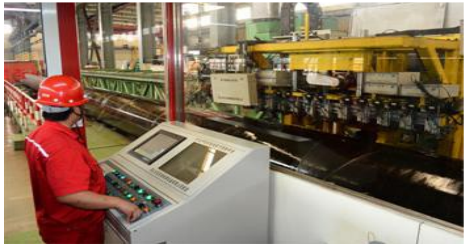
Hydrostatic Pressure Test
