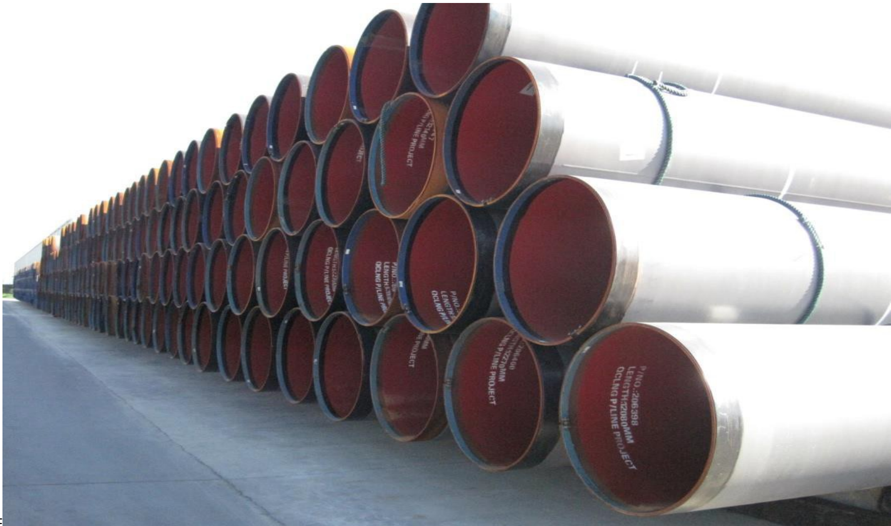
LIQUID EPOXY LINING+DOUBLE LAYER FBE COATING
