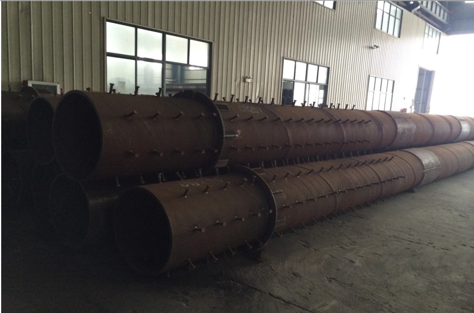
AS1163 C350L0 STUBBED PIPE PILING
